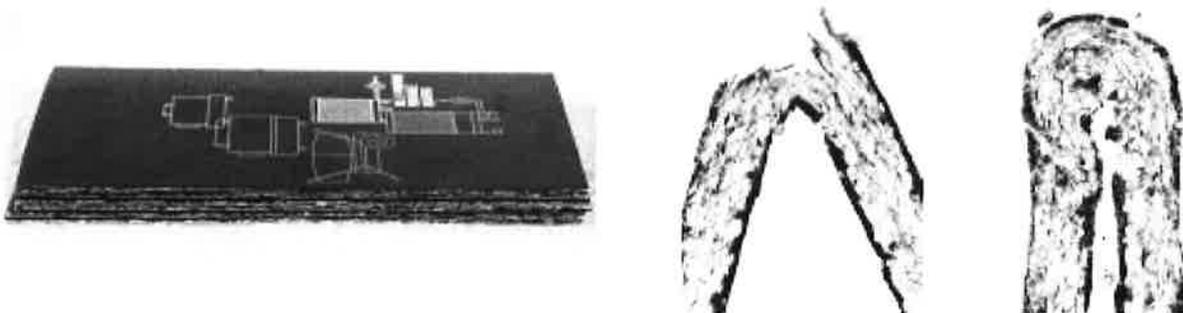
**Figure 7.** Fold cracking may occur when the paper is too dry. The moisture content of the sample in the center example was 20% RH; that on the right 50% RH.
