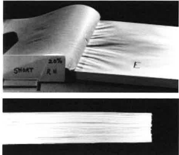
**Figure 5.** "Buckles" and "starts" occur with moisture changes in paper. "Buckles" shown on the top occur when paper is bound perpendicular to the grain; "starts" occur when bound parallel to the grain (bottom photo).
