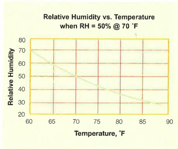
As the temperature of the air increases, its ability to hold moisture increases. Air, when heated, will retain the same absolute humidity, but its relative humidity will be lowered (**Figure 2**). Conversely, as the temperature of air decreases, its ability to hold moisture is reduced. Air when cooled therefore, also will retain the same absolute humidity, but its relative humidity will be increased.
